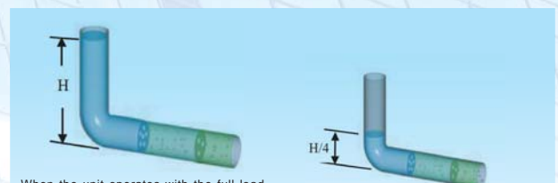
When the unit operates with half of the load, the liquid column height changes from H to H/4. Since the static pressure is insufficient, the amount of refrigerant passing the first orifice plate is half of that for the full load, reduction of the upstream volume leads to flash vaporization generated between the two orifice plates, a lot of flash gas mixed with liquid refrigerant passes through the second orifice plate, and the refrigerant volume is also reduced by one half accordingly.
